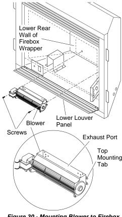
Figure 30 - Mounting Blower to Firebox
